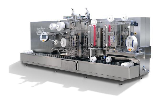
The **Natec FreePack 2000** machine produces individually-wrapped processed cheese slices (IWS) using a continuously operating production method.
